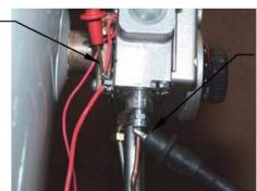
Alligator clip to copper sheath of thermocouple
