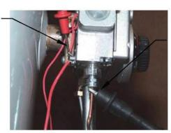
Alligator clip to copper sheath of thermocouple
