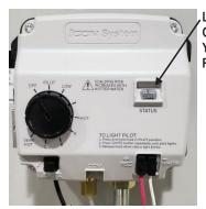
LED Colors: Green - Normal operation Yellow - Low thermopile voltage Red - Valve fault
