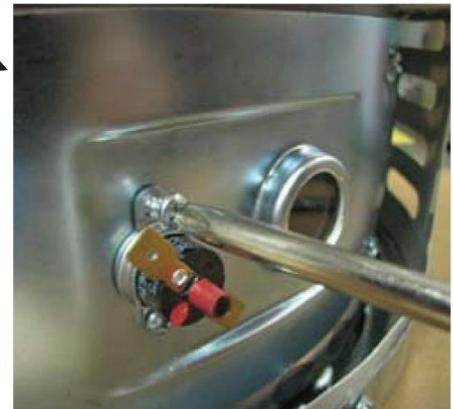
**NOTE:** Wire terminations are interchangeable with either resettable thermal switch connection.
