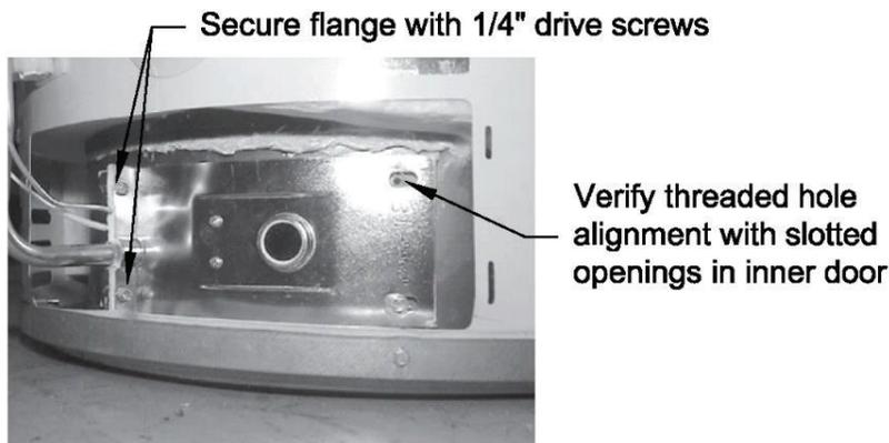
Step 10. Reconnect wire leads from the gas valve to resettable thermal switch (see Step 6 photo).
