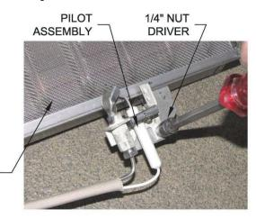
Step 4. With a multi-meter set to ohms setting, check continuity through igniter/flame sense wire. Replace pilot if no continuity.
