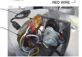
Step 14. Place the relay and its harness fully inside the damper housing.
