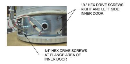
Step 15. Replace outer jacket burner access door.
