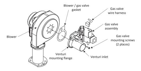
Step 8. Install new gas valve with new gasket provided. Secure gas valve in place using screws from step 6.
