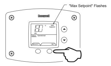
Step 3: Press the "UP" or "DOWN" buttons to change the maximum setpoint value. This will limit the maximum setpoint the user can select. Note: The maximum setpoint is approximately 180°F.
