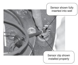
If sensor clip is damaged replace clip. Replace sensor if damaged.
