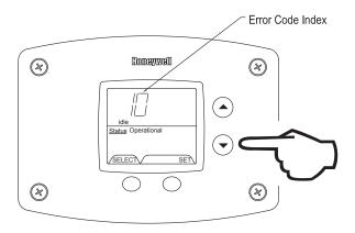
Step 3: Press the "Select" button to view the error code for "code 10". If there is a number displayed, note what the number is. The label next to the water heater display will identify the code number. If no number is displayed with only a "--" in the water heater display, then there has not been an error code for error code index 10.
