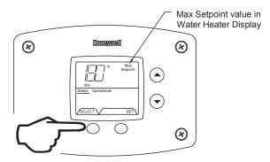
2. Tank Sensor Temperature Displayed Water Temperature Average.
