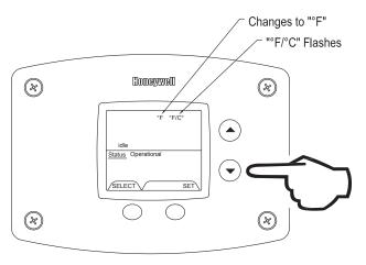
Step 4: Press "Set" button to confirm "F or "C format. "F/"C will stop flashing
