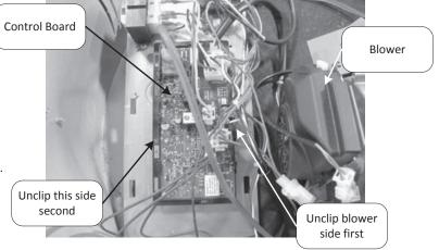
Step 5. Carefully disconnect all wire connections from control board.
