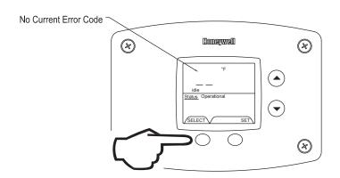
Step 2: Press the "Temperature Down" button to select the error code index, starting with the most recent error code "10".
