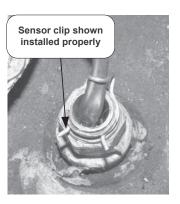
If sensor clip is damaged replace clip. Replace sensor if damaged.
