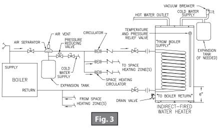
**Water Boiler Piping with Circulators**
