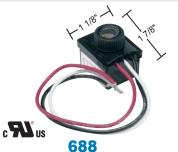
120V Button Photo Control 11/16" Dia. mounting hole required Up to 300W Inc., 54W LED 39W Fluor., 100W H.I.D. SPECIFY: Black
