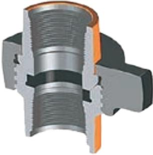
C&C's Figure 602 has a replaceable lip-type seal ring of Buna-N specifically designed to minimize fluid flow turbulence. The replaceable lip-type ring also provides a pressure seal and protection for the metal-to-metal seating surfaces. These unions are recommended for manifold and truck mounting where size and weight are critical. Recommended for air, water, oil, gas or mud service up to 6,000 PSI NSCWP.
