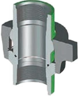
C&C's Figure 1003 (Mis-aligning Union) has NPT or Butt Weld Ends. It is constructed of Forged Alloy Steel, and comes with a Buna N O-Ring. Recommended for high pressure water, oil, mud or gas service where alignment of piping is a problem, with up to 7 1/2° angular adjustment from center (15° total).
