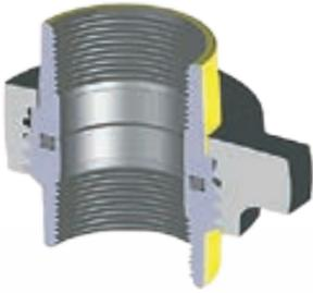
C&C's Figure 300 is manufactured from carbon steel. This Flat-Face type union has an O-Ring seal. Recommended for use where straight breakout of pipe segments is required. Suitable for water, oil, or gas service at pressures up to 12,500 PSI NSCWP. Please note that colors vary per pressure rating.
