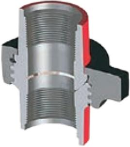
C&C's Figure 400 features a precision ball and cone sealing surface for sure metal-to-metal seal. Recommended for water, oil and gas service to 4,000 PSI NSCWP.
