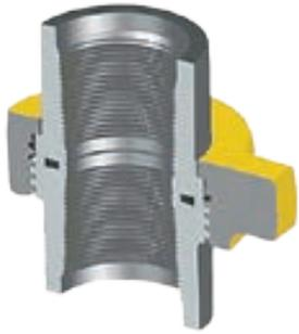
C&C's Figure 201 has EUE 8 Round Tubing Threads. This union is a Flat-Face type union that utilizes an O-Ring seal. The Figure 201 is available in 2 3/8" EUE and 2 7/8" EUE. Like parts in each size are interchangeable with other manufacturers' unions. Recommended for water, oil or gas service to 3,000 PSI NSCWP.
