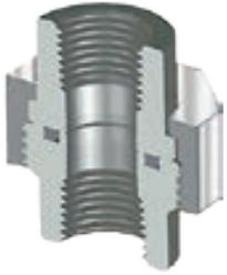
C&C's Figure OCT is manufactured from forged and normalized carbon steel to ASTM A105 with high speed ACME Threads. The Figure OCT is precision machined in dimensional compliance with MSS SP 83.
