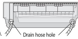
4. When extending the Drain Hose, hold the end of Drain Hose and Extended Hose, rotate and insert the drain hose into Extended hose for 1.57~1.77 inch(40~45 mm). Make sure the two hoses are firmly connected, there is no water leakage.
