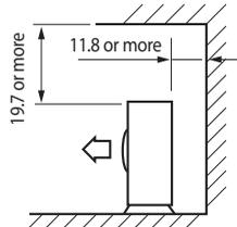
◆ When the walls are blocking front and the rear side of the outdoor unit
