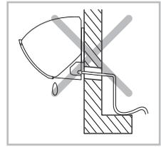
The drain hose must not be bent.
