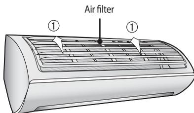
2. There's one hook in both side of the filter, press the surface of the Air filter softly and get the hooks into the main body. ②
