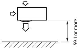
◆ When 3 sides of the outdoor unit are blocked by the wall
