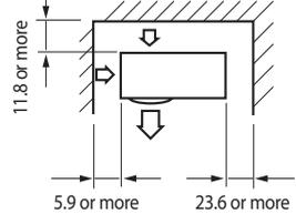
◆ The upper part of the outdoor unit and the air outlet is towards the wall
