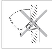
The drain hose must NOT slant upwards.
