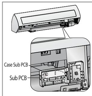
4. Find the PCB wire, and connect the wire to the Sub PCB as seen in the picture.
