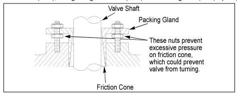
Figure 5 — Friction Cone Adjustment
