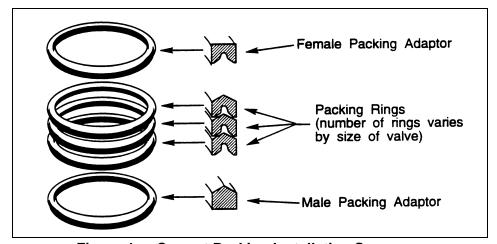
Figure 4 — Correct Packing Installation Sequence
