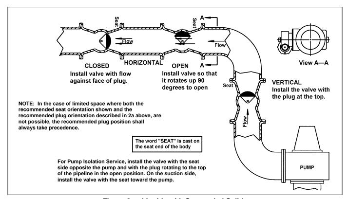
Figure 2 — Liquids with Suspended Solids
