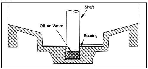
Figure 6 — Hydraulically Removing the Lower Bearing
