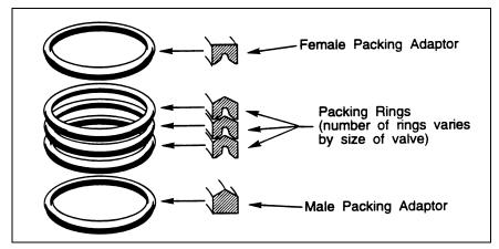
Figure 4 - Correct Packing Installation Sequence
