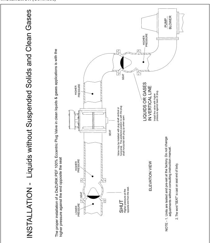
Figure 1—Liquids without Suspended Solids and Clean Gases
