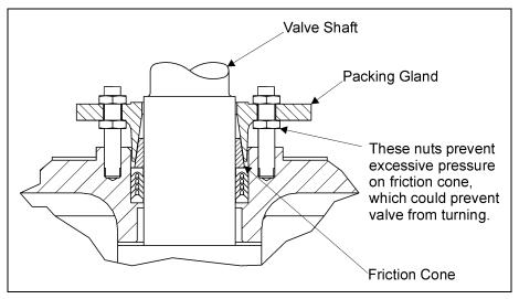
Figure 5—Friction Cone Adjustment
