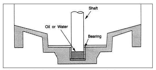
Figure 6—Hydraulically Removing the Lower Bearing in the Valve Body
