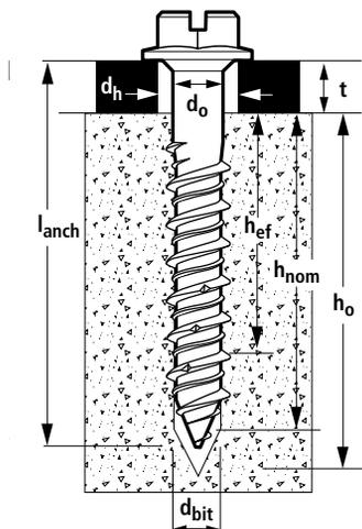
Slotted hex head version pictured, flat head length is measured from top of head to tip of anchor.
