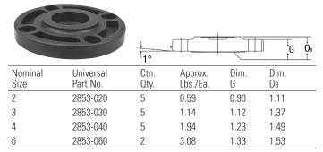
Note: One-piece webbed flanges have oblong bolt holes which permit mating with ANSI B16.5, 150 lb.; BS 1560, class 150; ISO 2084, PN10; and DIN 2532, PN10.
