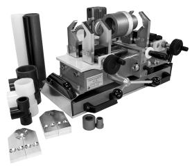
The bench-mount socket fusion machine is designed to join polypropylene and Kynar® PVDF IPS piping systems. Each machine, Models 7511XT, 3511, and 3600, is sized and specified to handle a particular range of IPS pipe sizes. Two clamps hold the pipe and one clamp holds the corresponding fitting or valve end connector in the precise position for socket fusion. Detailed operating instructions are found in the *Chemtrol Thermoplastic Piping Technical Manual*.
