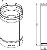
Galvanized outer jacket can be used as a conduit for single-wall PolyPro pipe. In exterior applications, provides protection from impact and UV light. Also provides some insulation value for use in colder climates. Can be field-painted if desired. Simple twist-lock assembly. To calculate installed length, subtract 1 1/2" for each joint. Includes internal metal support ring. PolyPro pipe sold separately.
