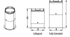
Adjustable Adapter with flange for galvanized outer jacket. Flange attaches to appliance cabinet with supplied screws. To calculate installed length, subtract 1 1/2" for each joint.
