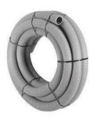
Use to line masonry chimneys that vent condensing appliances. Double-wall construction. Can be cut to precise length in the field. Available in 25, 35 or 50 foot lengths. 5" diameter flex comes in rolls of 98 feet only.
