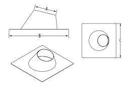
Use to weather-proof the penetration of the galvanized outer jacket through the roof. Made of galvalume.
