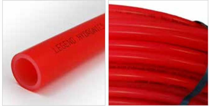
The externally extruded EVOH oxygen barrier reduces oxygen molecule permeation into the water. Compliant with standard DIN4756 (< 0.1 grams/m 2 /day).
