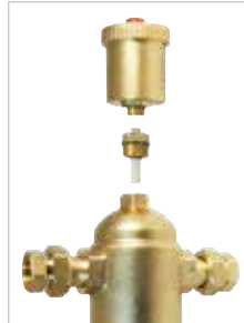
The automatic high capacity air vent attaches to the T-88 through a check valve to allow removal without system pressure loss.
