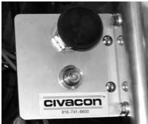
CCP-1 used as a Load Valve to release the Guard Bar Lock over APIs. Pop-Up confirms Vapor Vents are "open".
