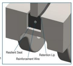
flows. Secondly, the seat is reinforced with a heavy stainless steel wire. The ends of the wire are wrapped around gland bolts. The wire adds rigidity to the seat form which also prevents seat movement during high flow or valve opening/closing operation.
