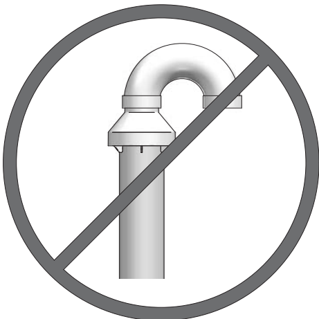
Figure 5-5 Do Not Install U-Bend to Rain Cap
