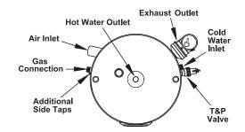
Top Outlet: 1" NPT Side Inlet: 1" NPT Side Taps: 1" NPT
