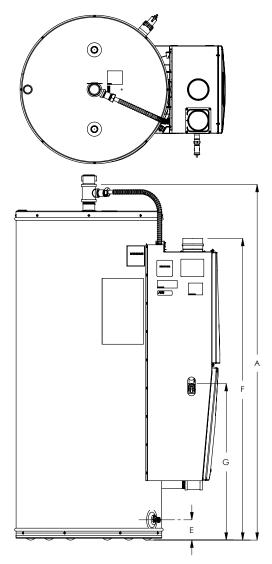
Water Connection Size: Inlet/Outlet 2" Female NPT Supply Gas Connection: 3/4" Male NPT
