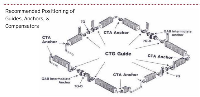
Expansion compensators must be both correctly selected and properly installed for effective performance in service. The reactions created by pressure and movement within the piping system should be carefully considered and the following precautions taken at installation:
