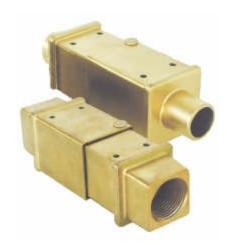
The heavy duty **Keflex<sup>TM</sup> 7Q Expansion Compensators** are specifically designed for high pressure service, available in sizes ¾" to 4", in both single and dual units. The single type is capable of absorbing 2" total movement, 1 ½" in compression and ½" in extension from the factory predetermined setting. The dual type will absorb 3" of pipe extension and 1" pipe compression for a full rated traverse of 4".
