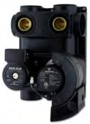
Flo-Link series foamed flow center with high impact polystyrene cabinet (shown with variable speed Grundfos Magna GEO pump): Flo-Link flow centers are available in one pump and two pump configuration with variable speed (UPS32-140) and constant speed (UP26-99, UPS26-99, or UP26-116) pump(s).
