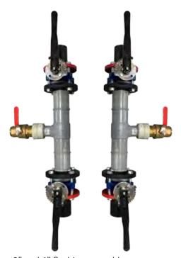
3" and 4" flushing assembly: PP-R body, HDPE fusion connections to/ from ground loop and building, 2" brass ball valve flushing connections, butterfly isolation valves (sold as a set, as shown)
