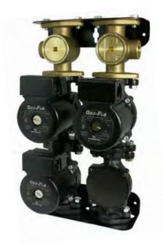
GPM series bracket style flow center: (Left is GPM-3; right is GPM-1 (also available as GPM-2, and GPM-4). Designed for Southern applications, where ground loop temperatures do not cause condensation.
