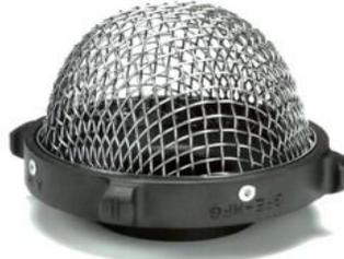
**A-LL Low Level Strainers** - Our low level strainer is essential for pumpers over 1200 gpm and delivers the maximum water available. A 45 degree elbow with a constant swiveling collar enables the strainer to sit flush in a porta-tank. The strainer is made of hardcoated high-strength extruded 6061-T6 aluminum alloy. Rounded base design ensures you can't snag the sides or bottom of your porta-tank. Please specify thread or storz size when ordering.
