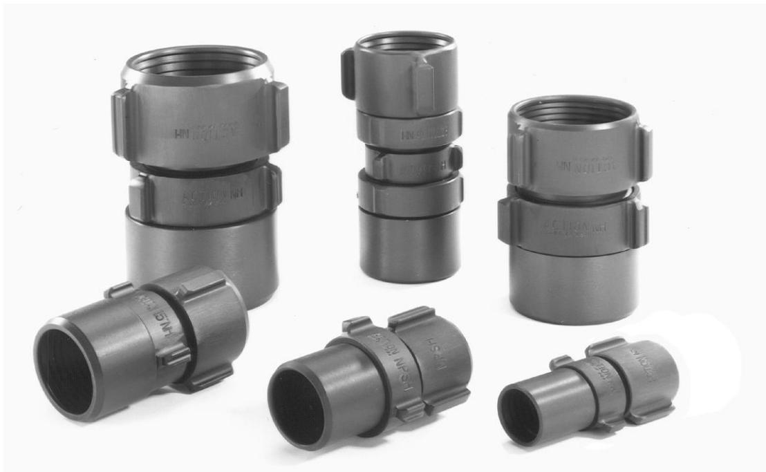
**A- Aluminum Couplings** - Hardcoated, heavy-duty, lightweight fire hose couplings are made from 6061-T6 high-strength aluminum alloy; complete with expansion rings and gaskets. Sold as complete sets but can order female or male only
