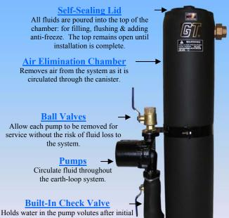
In the pump volutes after initial filling. This feature protects the pump by keeping water on the bearings even if the chamber runs dry.
