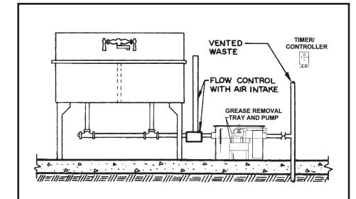
60100H-GRD Series Interceptor on floor, servicing a sink, shown installed with an optional -GRD Grease Removal Device.
