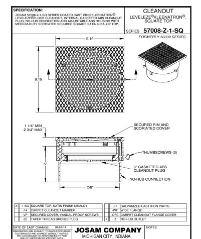
JOSAM 57008-Z-1-12 SERIES COATED CAST IRON KLEENATRON® LEVELEZE® FLOOR CLEANOUT, INTERNAL GASKETED ABS CLEANOUT PLUG, NO-HUB CONNECTION AND ADJUSTABLE ABS HOUSING WITH MEDIUM-DUTY SCORIATED SECURED ROUND SATIN NIKALOYTOP RECESSED FOR TILE.
