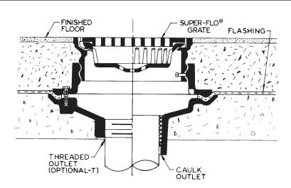
32100-AE-81 Series SUPER-FLO® Floor Drain shown installed in a poured concrete floor with floor finish. LEVELEZE® Adjustable Collar provides vertical adjustment, facilitating installation and forming a perfect surface between top of drain and floor finish.
