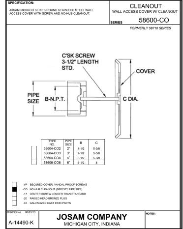
JOSAM 58600-COT SERIES ROUND STAINLESS STEEL WALL ACCESS COVER WITH SCREW AND NO-HUB CLEANOUT TEE.
