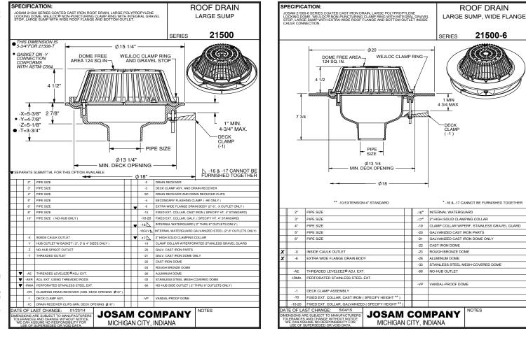
JOSAM 21500-AE SERIES COATED CAST IRON LEVELEZE® ROOF DRAIN, LARGE POLYPROPYLENE LOCKING DOME, WEJLOC® NON-PUNCTURING CLAMP RING WITH INTEGRAL GRAVEL STOP, BOLTED SUPPORT RING, ADJUSTABLE TOP, LARGE SUMP WITH WIDE ROOF FLANGE AND BOTTOM OUTLET.
