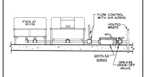
60115-SA Series Semi-Automatic shallow Interceptor installed on floor, servicing a double compartment sink and dishwasher.
