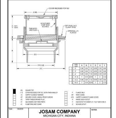
JOSAM 55000-1-13 SERIES COATED CAST IRON KLEENATRON® II LEVELEZE® FLOOR CLEANOUT, INTERNAL ABS CLEANOUT PLUG, ADJUSTABLE CAST IRON HOUSING WITH MEDIUM-DUTY SCORIATED SECURED ROUND SATIN NIKALOY COVER RECESSED FOR TERRAZZO FLOORING
