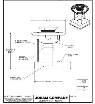
JOSAM SERIES 30000-ST COATED CAST IRON FLOOR DRAIN, TWO-PIECE BODY WITH DOUBLE DRAINAGE FLANGE, 1/2" PRIMER TAP WITH PLUG, WEJLOC INVERTIBLE CLAMP COLLAR THREADED FOR JOSAM ADJUSTABLE STRAINERS WITH SIDE OUTLET SHALLOW TRAP.
