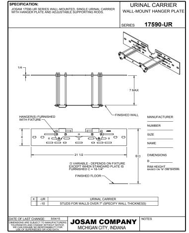
JOSAM 17590-DP SERIES WALL-MOUNTED, SINGLE URINAL CARRIER WITH HANGER PLATES AND ADJUSTABLE SUPPORTING
