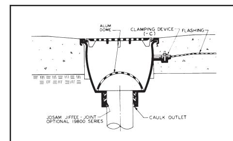
49580A-NB Series SUPER-FLO-SEPTOR® Floor Sink shown installed in a poured concrete floor on the ground level.
