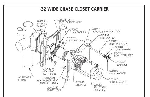
**SPECIFICATION:** JOSAM –32 coated cast iron Wide Chase Closet Carrier with adjustable closet connection, adjustable pylon feet, ABS extension with integral test cap, chrome plated trim, coated accessories and JIFFEE-SEAL Neoprene fixture gasket, for use with blowout or siphon jet water closets.
