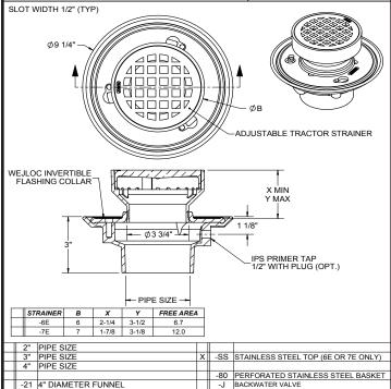
JOSAM 30000-S-SS-T SERIES TYPE 316 CAST STAINLESS STEEL FLOOR DRAIN, TWO-PIECE BODY WITH DOUBLE DRAINAGE FLANGE, WEJLOC® INVERTABLE FLASHING COLLAR, WEEPHOLES, BOTTOM THEADDED OUTLET CONNECTION AND ADJUSTABLE SQUARE SUPER-FLO® STRAINER.
