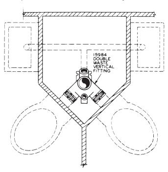
15984 SERIES DOUBLE WASTE VERTICAL FITTING SHOWN INSTALLED IN A TYPICAL ROOM BOTTOM DISCHARGE TOILET FACILITY LAYOUT
