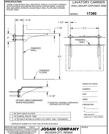
JOSAM 17390 SERIES WALL-MOUNTED, SINGLE LAVATORY CARRIER WITH EXPOSED ACID-RESISTING WHITE COATED ARMS, LEVELING AND SECURING SCREWS, ADJUSTABLE WALL PLATE, BACK PLATES AND CHROME PLATED TRIM.
