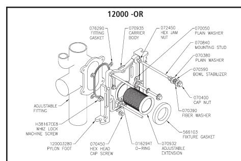
**SPECIFICATION:** JOSAM 12000-OR Series coated cast iron CHASE-SAVER® II Closet Carrier with adjustable connection, adjustable pylon feet, ABS extension with integral test cap, chrome plated trim, coated accessories and JIFFEE-SEAL Neoprene fixture gasket, for use with blowout or siphon jet water closets.
