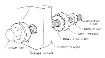
FH Hardware Part #: 565985T Mounting Stud and Back-up Nut not included in FH Hardware Kit.
