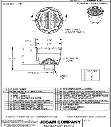
JOSAM 49580A-NB SERIES ROUND CAST IRON 8-1/4" DEEP SUPER-FLO-SEPTOR® FLOOR SINK WITH ACID RESISTING INTERIOR, DOUBLE DRAINAGE FLANGE WITH WEEPHOLES, BOTTOM OUTLET," ALUMINUM INTERNAL DOME STRAINER, NIKALOY SANITARY SLOPED RIM AND NIKALOY LIGHT-DUTY SUPER-I-LOW ANTI-TILTING GRATE.
