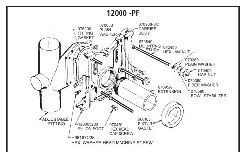
**SPECIFICATION:** JOSAM 12000-PF Series coated cast iron CHASE-SAVER® II Closet Carrier with adjustable connection, adjustable pylon feet, ABS extension with integral test cap, chrome plated trim, coated accessories and JIFFEE-SEAL Neoprene fixture gasket, for use with blowout or siphon jet water closets.
