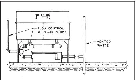
60115A Series Interceptor installed on floor under sink. (Recommended only if there is adequate head room for cover removal and service.)
