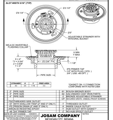
JOSAM SERIES 30000-D CAST IRON FLOOR DRAIN, TWO-PIECE BODY WITH DOUBLE DRAINAGE FLANGE AND 1/2" PRIMER TAP, WEJLOC ◎ INVERTIBLE FLASHING COLLAR, WEEPHOLES, BOTTOM OUTLET CONNECTION AND NIKALOY ADJUSTABLE DOME STRAINER.
