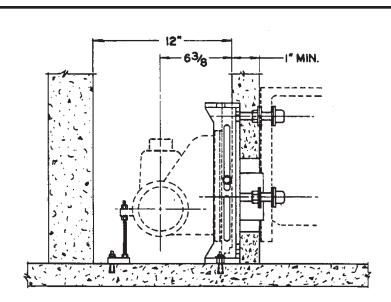
Installation of 12000-PF Series Adjustable Carrier in a standard 12" wide pipe chase showing minimum extension.
