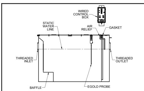
60210A-EGOLD Series Interceptor with factory installed Josam EGOLD-1000 Electronic Grease/Oil Level Detector for installation in high volume applications such as hotels, hospitals and schools.
