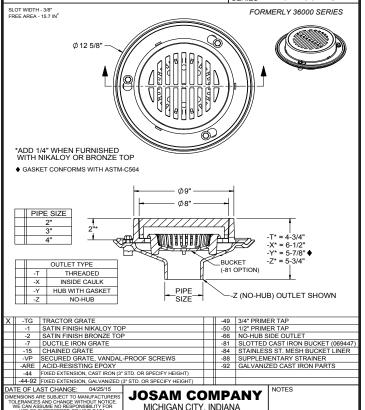
JOSAM 32150 SERIES COATED CAST IRON FLOOR DRAINS, TWO-PIECE BODIES WITH DOUBLE DRAINAGE FLANGE, WEEPHOLES, BOTTOM OUTLETS, 9" ROUND TOPS, ONE BODY FURNISHED WITH A SOLID BRONZE PLUG, OTHER BODY FURNISHED WITH AN EXTRA-HEAVY, ANTI-TILLTING, SUPER-FLO® GRATE WITH PERIMETER DRAINAGE SLOTS.
