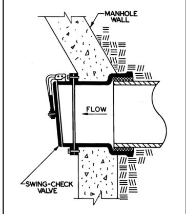
67800 Series swing-check Backwater Valve shown installed in a manhole terminal.
