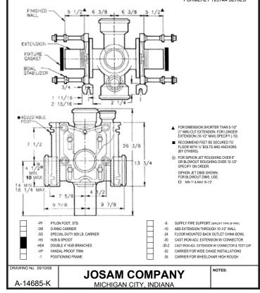
JOSAM 14004 SERIES COATED CAST IRON SINGLE VERTICAL 4" HUB AND SHOOT LETT-HAND OFFSET FITTING WITH 2" HUB VENT ADJUSTABLE CARRIER BODY, INVERTIBLE FOR SIPHON JET OR BLOWOUT CLOSETS, WITH ABS EXTENSION WITH INTEGRAL TEST CAP PYLON FEET, PLATED HARDWARE AND NEOPRENE FIXTURE GASKET.
