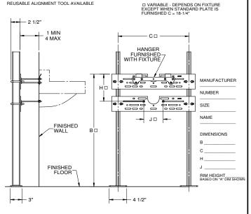
RECOMMEND ALL FEET BE SECURED TO FLOOR WITH 1/2" BOLTS AND ANCHORS BY OTHERS.
