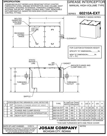
JOSAM 60210A-ISI SERIES ACID RESISTANT EPOXY COATED FABRICATED STELL GREASE INTERCEPTOR, HIGH VOLUME, THREADED CONNECTIONS, INTERNAL AIR-RELIEF, VISIBLE DOUBLE WALL TRAP, INTEGRATED SOLIDS INTERCEPTOR, GASKETED NON-SKID COVER AND FLOW CONTROL FITTING.
