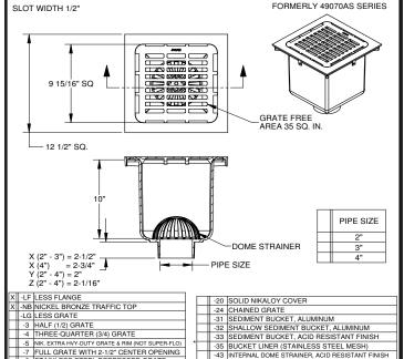
STAINLESS STEEL DEPRESSED GRATE -45 LESS INTERNAL DONE STRAINER -VP SECURED GRATE, VANDAL-PROOF SCREWS -55 1/2" PRIMER ADAPTER, 88450 PROVIDED -15 STAINLESS STEEL RIM & GRATE -X INSIDE CAULK OUTLET -16 GRATE WITH 4" ROUND FUNNEL
