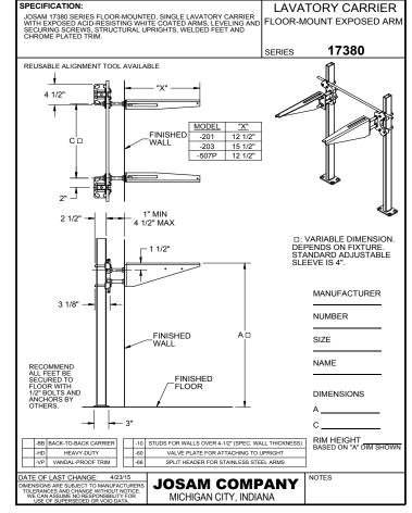
JOSAM 17380-BB SERIES FLOOR-MOUNTED, BACK-TO-BACK LAVATORY CARRIER WITH EXPOSED ACID-RESISTING WHITE COATED ARMS, LEVELING AND SECURING SCREWS, STRUCTURAL UPRIGHTS, WELDED FEET AND CHROME PLATED TRIM
