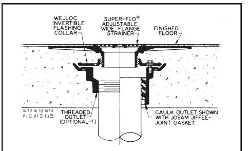
30000-WF6S Series SUPER-FLO® Adjustable Strainer Floor Drain shown installed in a composition deck floor. Wide flange assures that bonding of floor material is watertight and permanent.
