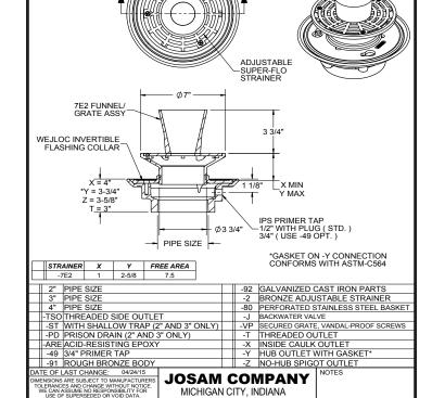
JOSAM 30000-23 SERIES CAST IRON FLOOR DRAIN, TWO-PIECE BODY WITH DOUBLE DRAINAGE FLANGE AND 1/2\* PRIMER TAP, WEJLOC\* INVERTIBLE FLASHING COLLAR, WEEPHOLES, BOTTOM OUTLET CONNECTION AND NIKALOY ADJUSTABLE ROUND STRAINER WITH OVAL FUNNEL.
