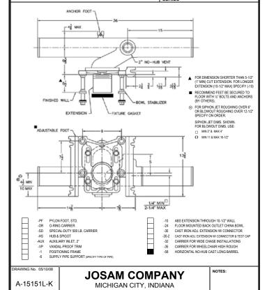
JOSAM 12684 SERIES COATED CAST IRON SINGLE HORIZONTAL 4" NO-HUB RIGHT-HAND OFFSET FITTING WITH 2" NO-HUB VENT AND ADJUSTABLE CARRIER BODY, INVERTIBLE FOR SIPHON JET OR BLOWOUT CLOSETS, WITH ABS EXTENSION WITH INTEGRAL TEST CAP, PYLON FEET, ANCHOR FOOT, PLATED HARDWARE AND NEOPRENE FIXTURE GASKET
