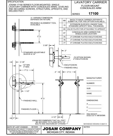
JOSAM 17100-BB SERIES FLOOR-MOUNTED BACK-TO-BACK LAVATORY CARRIER WITH CONCEALED ARMS, LEVELING AND SECURING SCREWS, STRUCTURAL UPRIGHTS AND WELDED FEET.
