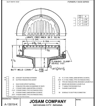
JOSAM 32100-SS-AE SERIES TYPE 316 CAST STAINLESS STEEL LEVELEZE® FLOOR DRAIN, DOUBLE DRAINAGE FLANGE, WEEPHOLES, ROUND TOP, ADJUSTABLE COLLAR WITH ROLLED THREADS AND HEAVY-DUTY LOOSE-SET ANTI-TILTING SUPER-FLO® GRATE WITH PERIMETER DRAINAGE SLOTS, BOTTOM OUTLET, BUTT WELL CONNECTION FOR SCHEDULE 40 PIPE.
