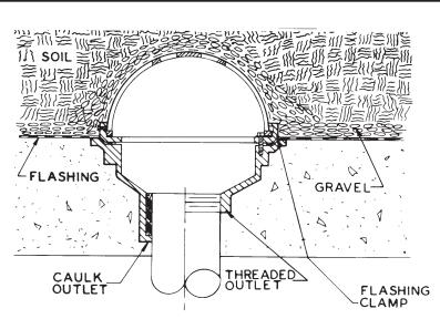
39600 Series Planting Area Drain shown in a typical installation providing drainage for an indoor planting area. Stainless mesh screen covered dome prevents entrance of dirt and gravel at the base of the planting area.
