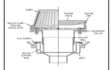
The adjustable integral top is mated to the body and support ring with a heavy machined thread which permits virtually unlimited top level adjustment to accommodate various deck thicknesses. The line contact between the threads provides positive circumferential support of the top at any adjusted elevation.
