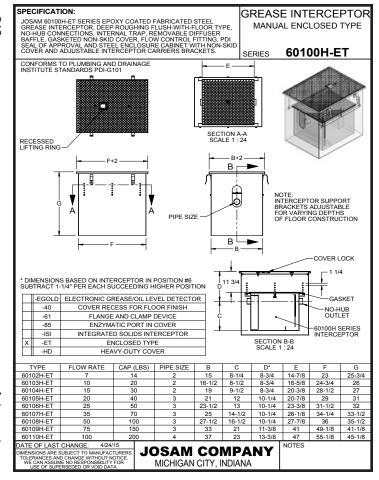
JOSAM 60:00H.RT SERIES EPOXY COATED FABRICATED STEEL GREASE INTERCEPTOR. DEEP ROUGHING FLUSH-WITH-FLOOR TYPE, NO-HUB CONNECTIONS, INTERNAL TRAP, REMOVABLE DIFFUSER BAFFLE, GASKETED NON-SKID COVER, FLOW CONTROL FITTING, PID SEAL OF APPROVAL AND STEEL FRAME WITH NON-SKID COVER AND ADJUSTABLE INTERCEPTOR CARRER BRACKET.
