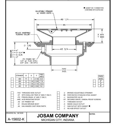
JOSAM 30000-M SERIES CAST IRON FLOOR DRAIN, TWO-PIECE BODY WITH DOUBLE DRAINAGE FLANGE AND 1/2" PRIMER TAP, WEJLOC® INVERTIBLE FLASHING COLLAR, WEEPHOLES, BOTTOM OUTLET CONNECTION AND CHROME PLATED ADJUSTABLE STANDPIPE WITH DOME
