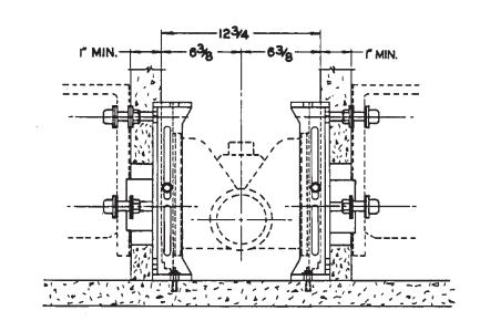
Installation of back-to-back 12000-PF Series Adjustable Carrier showing minimum extension.
