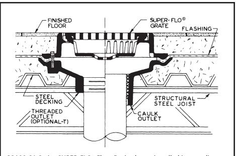
32100-81 Series SUPER-FLO® Floor Drain shown installed in a medium-duty single-pour concrete floor supported by steel construction.
