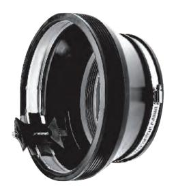
There is no substitute for the "standard boot" connector. Unlike any compression connector, "standard boots", with their mechanical connection to the pipe, will tolerate pipe deflections associated with flexible pipe and the O.D. variations common in rigid pipes. Connectors other than "standard boots" push the limits of what can be expected of the manhole and of the pipe at their connection.
