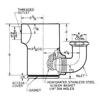
NOTE: 6" MIN. CLEARANCE REQUIRED BELOW COVER FOR REMOVAL OF BASKET.
