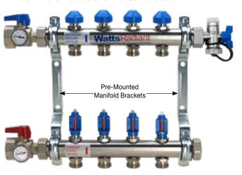
Matching fittings and accessories are made of solid brass and heavily plated with nickel to match the appearance of the manifold trunk. Standard features include flow balancing valves and flow meters on each circuit. Manifolds are sold in pre-mounted pairs.
