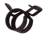
**SelfTite™ Clamps** — Pretensioned for easy field installation. The chrome-vanadium spring steel maintains a constant tension on the Onix under all operating conditions. SelfTites incorporate a zinc coating to guard against corrosion.
