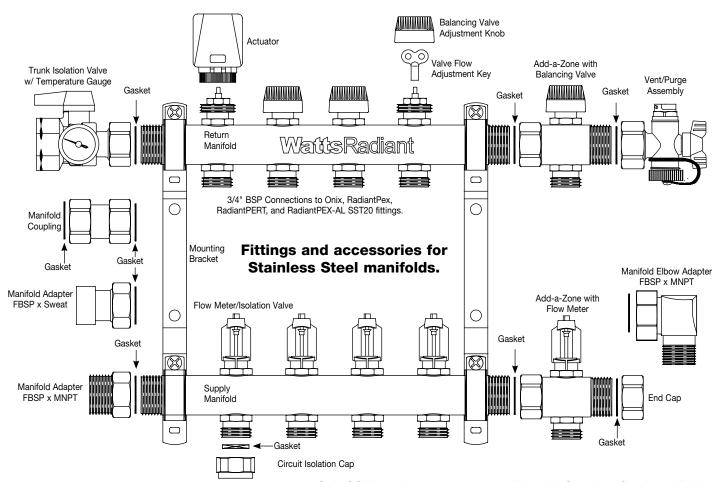
Only SST20 style parts are compatible with Stainless Steel manifolds.
