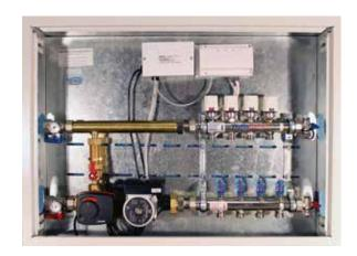
The ThermalPro Isotherm Mixing Module is a compact, prepiped, pre-wired pump and mixing valve control connected directly to a Watts 1" Standard or 1-1/2 Hi-Flow Stainless Steel manifold and installed in a white powder coated steel cabinet with cover door.
