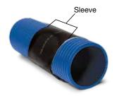
**R-flex Jacket Repair Sleeve** — To repair accidental damage to R-flex outer cover. Slide the sleeve over damaged area and heat with heat gun.
