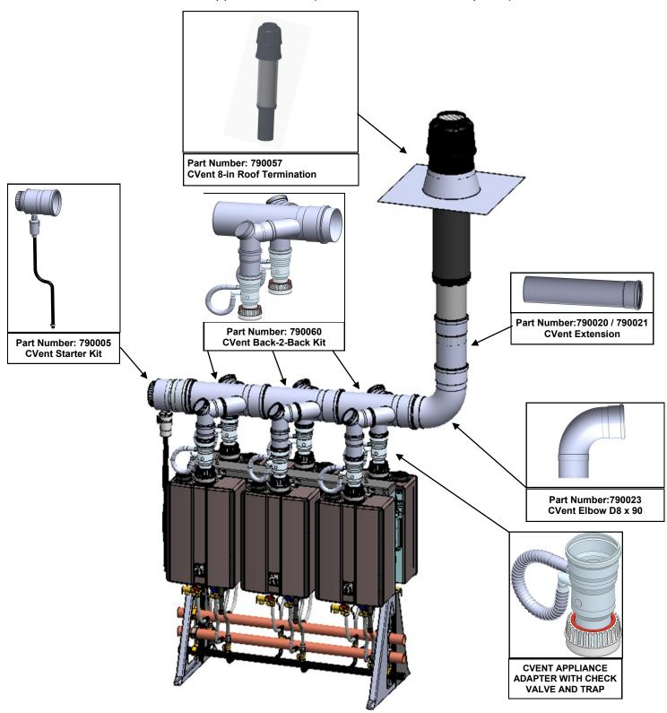
Complete Header Kit (B-to-B): U.S.-CV8BB6USRA Canada-CV8BB6CARA Complete Header Kit (In-line): U.S.-CV8IL3USRA Canada-CV8IL3CARA Vent termination per ANSI Z223.1/NFPA 54. For clearances not specified in ANSI Z223.1/NFPA 54, clearances are in accordance with local installation codes and the requirements of the gas supplier.
