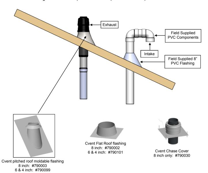
Vent termination per ANSI Z223.1/NFPA 54. For clearances not specified in ANSI Z223.1/NFPA 54, clearances are in accordance with local installation codes and the requirements of the gas supplier.
