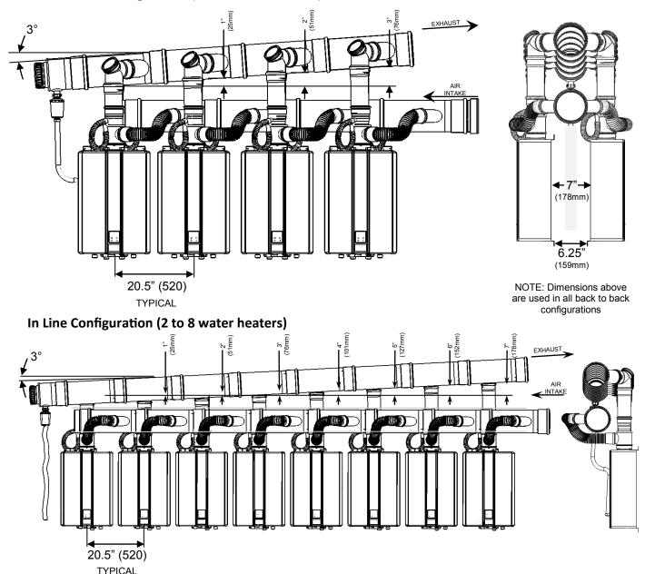
Note: If water heaters are mounted directly on a wall, air intake piping will need to be in front of the appliance adapters. The intake header in the drawing above has been removed for illustration purposes.
