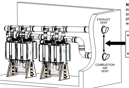
**NOTE:** During colder weather when the exhaust temperature is much hotter than the outside air, the exhaust fumes condense producing water vapor. As a result a plume of water vapor may be seen leaving the exhaust.
