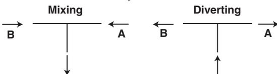
For normally open, reverse pipe A and B ports. B port is normally closed.
