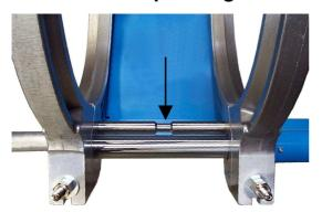
There is a tear-off bar mounted between the movable and the fixed clamping shells on the basic machine. It prevents the heating element from sticking to the heated-up pipe ends
