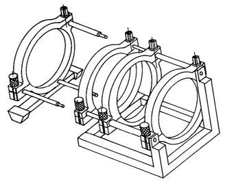
Dismantling of the outer fixed clamping device
