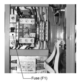
The control unit does **not** function although the control unit is connected to the power supply, the main switch is on, and the Emergency-Stop has **not** been pressed and locked.
