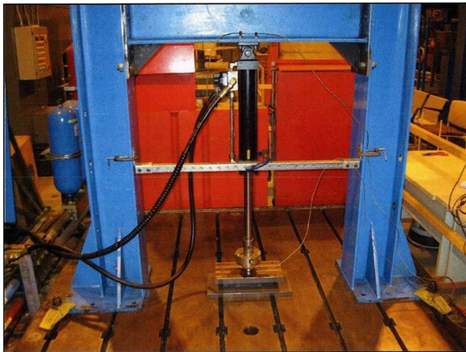
Figure 2: Compression durability test set-up – General view
