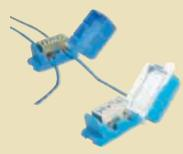
The **DryConn 3-way Direct Bury Lug** eliminates the need to cut the main line and installs in less than a minute. This connector is pre-filled with dielectric silicone sealant that never hardens making it waterproof and corrosion proof. The improved outer lid locks down in three places keeping your connection free from contaminants and the user friendly design prevents cuts and handling discomfort.
