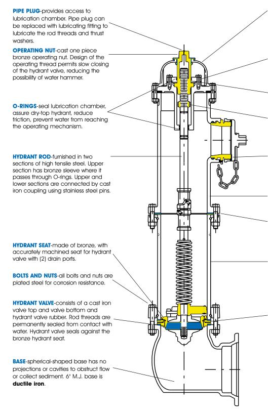
**WEATHER COVER** (cast iron with rubber weather shield)-The word "open" and an arrow show direction to turn the operating nut. The rubber weather shield prevents water and debris from entering the housing area.
