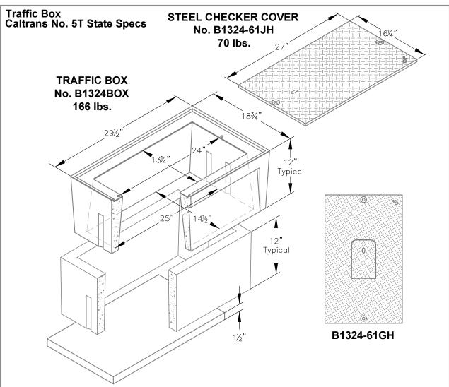
A high density reinforced concrete box with non—settling shoulders positioned to maintain grade and facilitate back filling. Approximate dimensions and weight shown.
