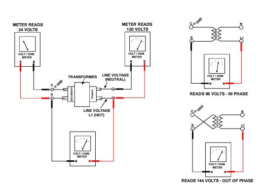
If meter reads approximately 96 volts - the primary to secondary are in phase - if reads approximately 144 volts out of phase - reverse low voltage wires.
