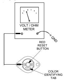
**Checking Flame Rollout Switch**
