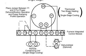
Two-Stage Heating with Single-Stage Cooling
