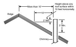
Termination More Than 10 Feet From Ridge, Wall or Parapet
