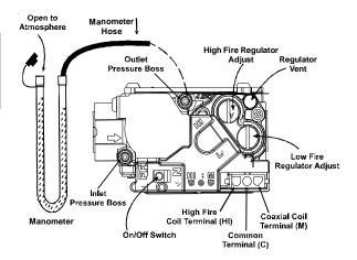
Measuring Manifold Gas Pressure (36G54 Valve)
