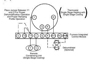
Single Stage Heating with Single Stage Cooling
