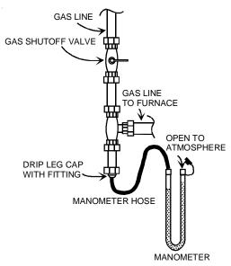
**Measuring Inlet Gas Pressure** (Alternate Method)
