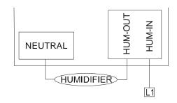
Wiring Using HUM IN - HUM OUT Terminals
