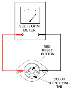
Testing Auxiliary Limit Control (80% & 90% Furnaces)
