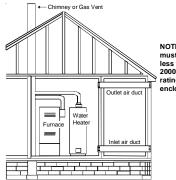
NOTE: The air duct openings must have a free area of not less than one square inch per 2000 BTU of the total input rating of all equipment in the enclosure\*.
