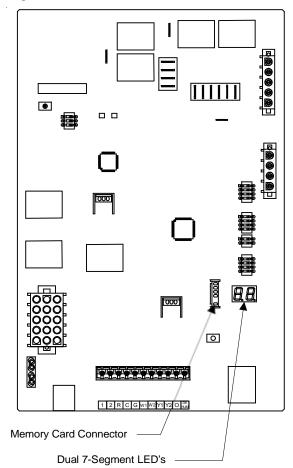
Internal Control Failure with Integrated Ignition Control. Check for voltage to the furnace and low voltage at the control board. Check for blown fuse on the control board. If the control determines it has an internal fault, it enters a locked-out state. Any of the situations mentioned will cause the dual, 7-segment LED's to be off. The control board should only be replaced only after all other checks from the *Troubleshooting Chart - ComfortNet™* have been verified.
