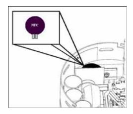
Inspect the large capacitors inside the control/end bell (see figure below). Replace the control/end bell if any of the capacitors are bulging or swollen.
