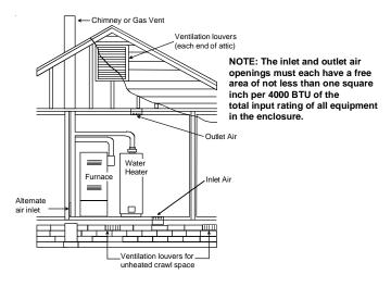
Figure A.9.3.3.1(1)(a) All Combustion Air From Outdoors -Inlet Air from Ventilated Crawl Space and Outlet Air to Ventilated Attic.
