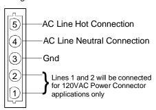
POWER CONNECTOR (1/2 HP MOTORS) "Motor Half" (Viewed from Plug End)
