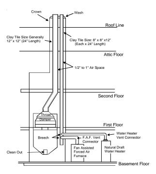
Typical Multiple Flue Clay Tile Chimney
