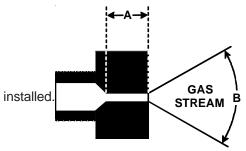
The length of Dimension "A" determines the angle of Gas Stream "B".
