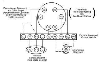
Two-Stage Heating with Two-Stage Cooling
