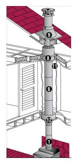
Interior installation on a wood stove using a finishing support.
