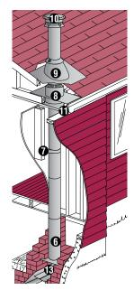
Chimney installed on a masonry fireplace.
