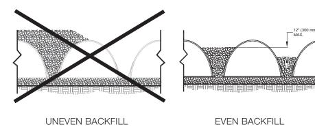
Backfill chambers evenly. Stone column height should never differ by more than 12" (300 mm) between adjacent chamber rows or between chamber rows and perimeter.
