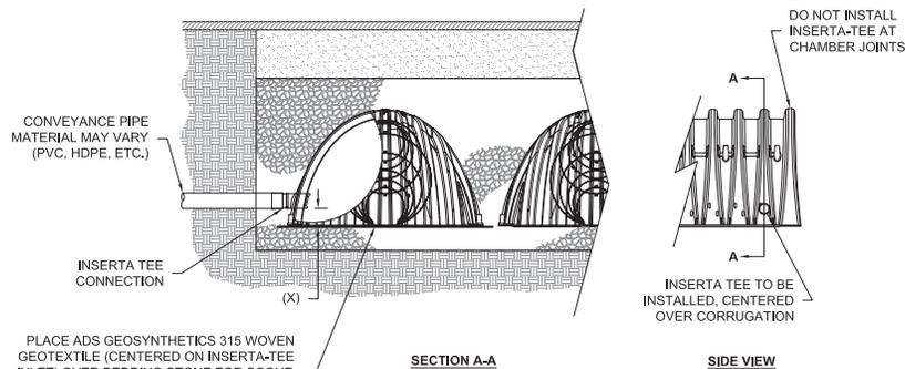
PLACE ADS GEOSYNTHETICS 315 WOVEN GEOTEXTILE (CENTERED ON INSERTA-TEE INLET) OVER BEDDING STONE FOR SCOUR PROTECTION AT SIDE INLET CONNECTIONS. GEOTEXTILE MUST EXTEND 6" (150 mm) PAST CHAMBER FOOT
