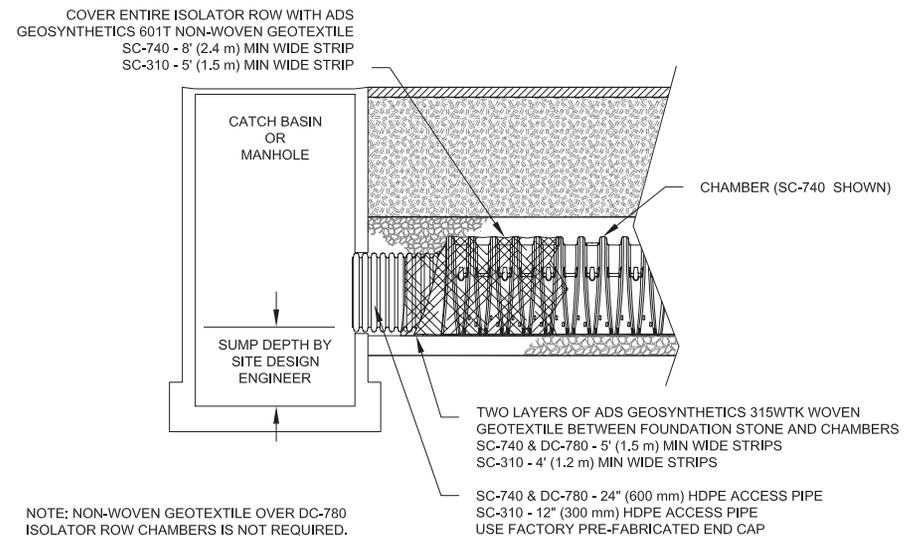
TWO LAYERS OF ADS GEOSYNTHETICS 315WTK WOVEN GEOTEXTILE BETWEEN FOUNDATION STONE AND CHAMBERS SC-740 & DC-780 - 5' (1.5 m) MIN WIDE STRIPS SC-310 - 4' (1.2 m) MIN WIDE STRIPS
