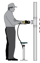
Simply thread into test tee and inflate (for maximum sealing performance, apply thread seal tape to the threads before use).
