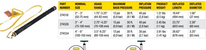
Long Test-Ball<sup>®</sup> & MS2<sup>®</sup> Long Test-Ball<sup>®</sup> plugs seals lateral during sewer air test
