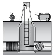
Attach Jet-Ball<sup>™</sup> to tag line and inflate
