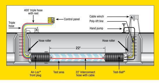
STAY OUT OF THE DANGER ZONE DURING THE TEST!! ALWAYS BLOCK PLUGS WHEN CONDUCTING AIR TESTS.
