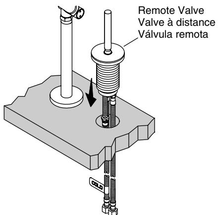
Insert the remote valve through the surface material.
