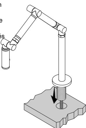
**4** Partially thread the screws into the ring.
