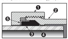
Threaded end-nuts (1) screw onto the threaded body (2), compressing the gaskets (3) against the pipe (4) to make a flexible, bottle-tight seal. Note the heavy body construction and ample seating area of the resilient gasket. Note also the manner in which the gasket is confined and protected from damage by the retainer ring (5).
