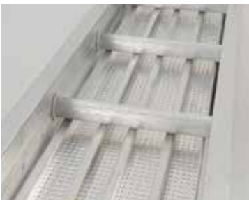
Rungs located on 12" centers for extra strength. The larger planks have lower rungs to prevent racking and buckling. These rungs also provide for a greater load-bearing area.
