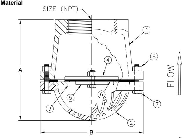
Max Temp 80°F (27°C) Max Pressure 75psi (15bar)
