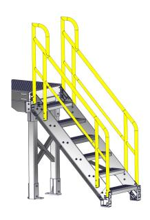
When tower and stairs are both used at the end of a platform, omit indicated hardware from tower assembly. These bolts will interfere with top step of stair unit.
