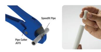
To prevent damage to the O-ring remove all burrs and sharp edges. When using Speedfit® or other types of PEX Pipe, we recommend the use of Pipe Insert.
