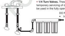
• 1/4 Turn Valves. These valves have been designed to allow temporary servicing of downstream equipment and must only be used in the fully open or fully closed position.
