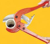
Position pipe in the cutter and close handles together to engage ratchet. Blade begins to cut on contact.
