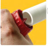
Use inside/outside Deburring Tool [Uniweld Part# 70079] to remove burrs from pipe.
