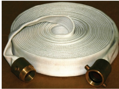
Double Jacket 800psi Test Service Test 400psi Working Pressure 270psi
