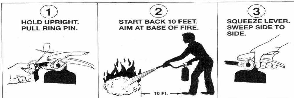
All **Croker** hand portable extinguishers comply with the recommendations of the National Fire Protection Association adopted by Underwriters Laboratories, that all hand portable extinguishers are rated 2A and/or 20B or higher be equipped with discharge hose and horn. In addition all 2A or higher A rated extinguishers have a minimum discharge time of 13 seconds.
