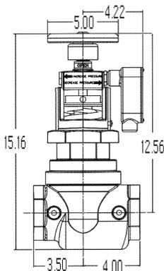
400LB. Field adjustable pressure regulating valve for use as a fire hose rack assembly valve or sprinkler control valve where pressure require regulation. Tampered resistant protective shroud. Both sides drilled and tapped 1/4" NPT.
