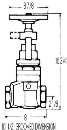
400LB. Field adjustable pressure regulating valve for use as a fire hose rack assembly valve or sprinkler control valve where pressure require regulation.
