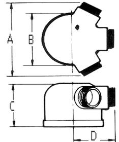
Cast Brass - Straight Pattern - IPT or Hose Thread Outlets
