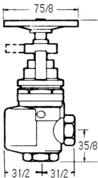
400 LB. Field adjustable automatic pressure regulating valve for use as a fire hose rack assembly valve or sprinkler control valve where pressures require regulation.
