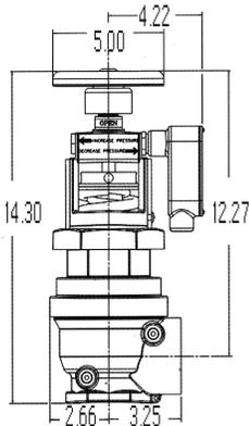
400 LB. Field adjustable automatic pressure regulating valve for use as a fire hose rack assembly valve or sprinkler control valve where pressures require regulation. Tamper resistant protective shroud. Both sides drilled and tapped 1/4" NPT.
