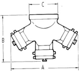
An exposed auxiliary inlet connection with 750 G.P.M. inlet capacity to supplement fire protection water supply. Exposed design provides and economical method of satisfying Fire Dept. inlet requirements.
