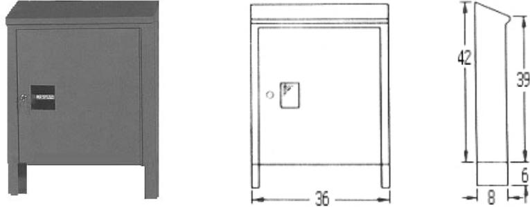
**1950** Marina cabinets will accommodate 1 1/2" Fire Hose Rack assembly with lined hose and a portable fire extinguisher.
