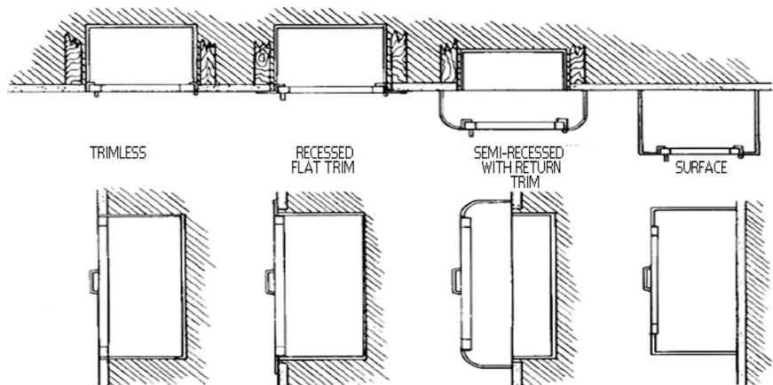
**For Use With 1 1/2" Fire Hose Rack Assembly & 2 1/2" Fire Dept. Valve**
