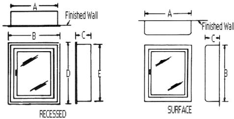
All Series **Recessed** cabinets are two-piece construction with adjustable screws for attachment of door and frame to tub. Pull handle with roller catch and continuous hinge with brass pin are standard hardware.
