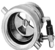
Restricts water pressure at hose line. A removable breakable link permits adjustment of restriction. Installed on bottom of rack nipple or on male side of FD valve.
