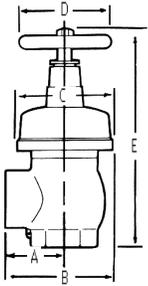
300lb. Non-adjustable automatic pressure regulating valve for use as a hose outlet valve or fire hose rack valve where inlet pressures require regulation. Figure No. 5555 may also be used as a zone control valve on a sprinkler system for flows up to 250 GPM.
