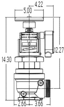
400LB. Field adjustable pressure regulating valve for use as a hose outlet valve where inlet pressures require regulation. Tamper resistant protective shroud. Both sides drilled and tapped 1/4" NPT.
