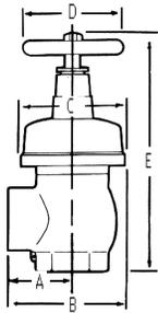
400lb. Non-adjustable automatic pressure regulating valve for use as a hose outlet valve or for hose rack valve or sprinkler control where inlet pressures require regulation.
