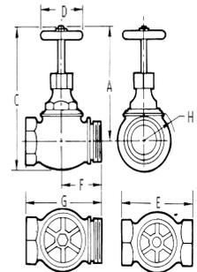
**STANDARD EQUIPMENT:** Female NPT inlet and outlet, cast brass with wheel handle. 300 PSI.
