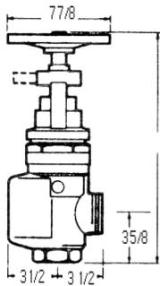
400LB. Field adjustable pressure regulating valve for use as a hose outlet valve where inlet pressures require regulation.
