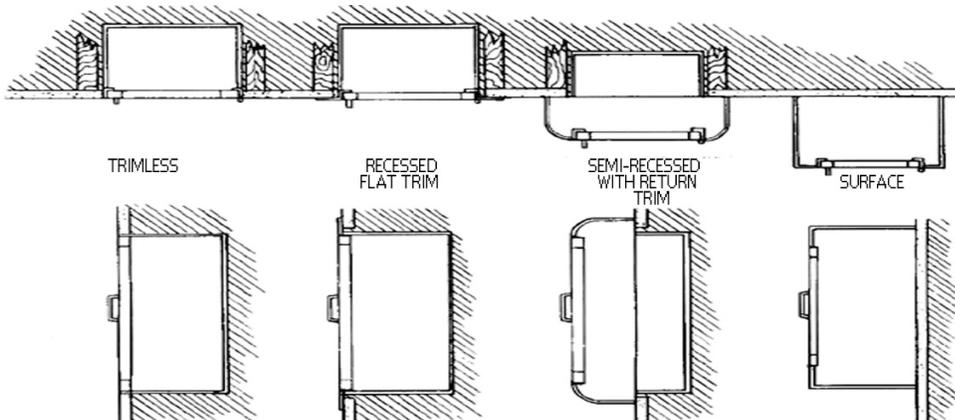
**For Use With Fire Dept Valve, 2 1/2" Fire Dept Valve & Fire Extinguisher**
