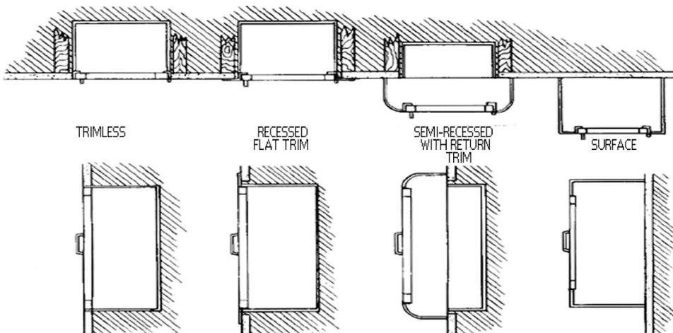
**For Use With Fire Hose Rack Assembly & Fire Extinguisher & Fire Dept Valve**
